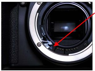
Step 3. Place the tape provided with the kit on the screw to prevent loosening of the screw due to vibration.
