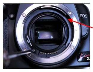
Step 2. Set the filter holder ring in place and replace the screw removed in step 1.
