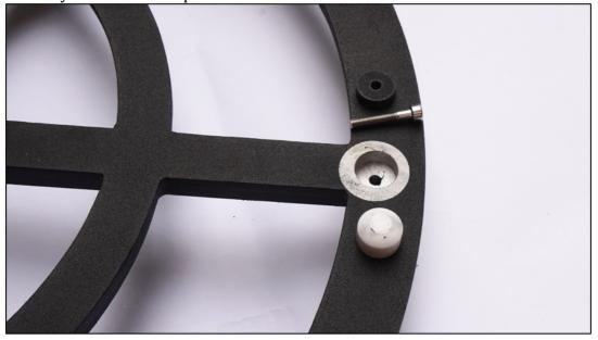
Insert the spacer, then the Teflon cylinder and fix it with the screw. Note: please do not tighten the screw too much or the thread may get damaged.
