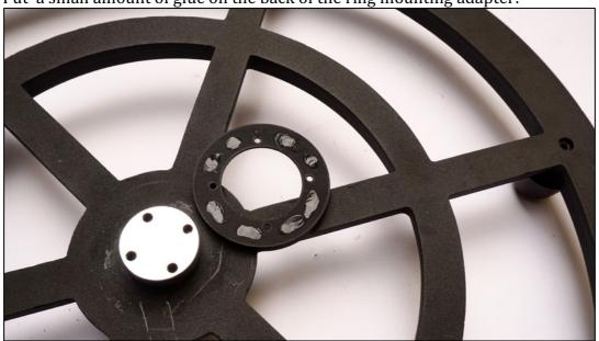
And put the adapter on the ground board (you may need to clean the surface with isopropyl alcohol or similar before this):
