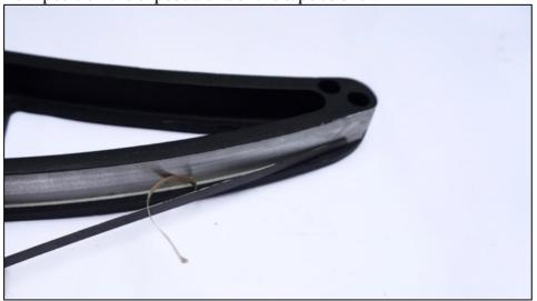
Use the soft cloth to put pressure on the tape and work your way until the end of the bearing – please apply plenty of pressure to avoid any air bubbles between the tape and the bearing:
