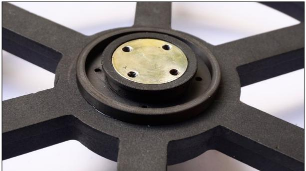
Please rotate the adapter back and forward a bit to distribute the glue uniformly.
