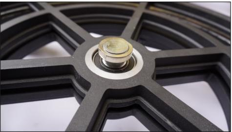
2. Now flip the ground board with the virtual rocker box around. Please remove four screws holding the pivot bolt using 5mm Allen key:
