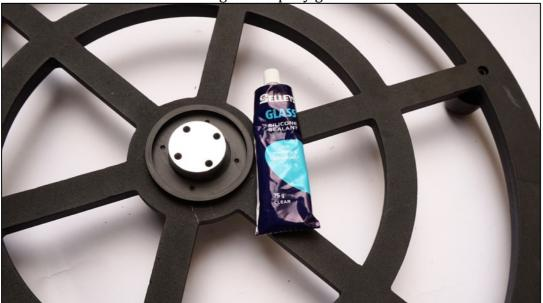
Put a small amount of glue on the back of the ring mounting adapter:
