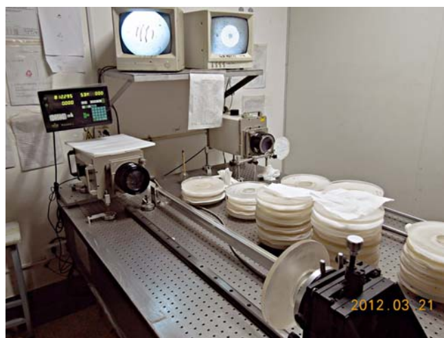
Figure 10. We test all of our primary mirrors on an optical bench by means of laser interferometry. In the picture, stacks of polished primary mirrors await testing on one of our optical test benches.
