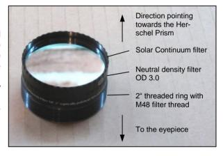
For changing filters unthread the 2" Click Lock® clamp from the prism body. Now seperate the connecting threaded ring 2"/M48. This ring serves as connecting element to attach the 2" Click Lock® clamp onto the prism body and additionally as filter holder for one or two standard 2" filters.
