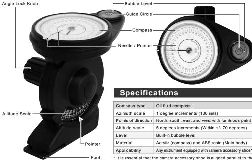
\* It is essential that the camera accessory shoe is aligned parallel to the optical axis of the camera's lens or corresponding equipment.
