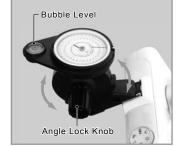
♠ On the altitude scale the angle is indicated by the pointer. The altitude is scaled in 5 degree increments.
