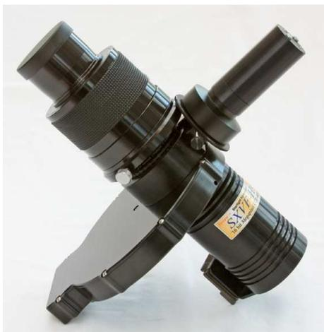
With this in mind, I tested the Filter Wheel/OAG combination with my William Optics FLT98 refractor using the 2" nosepiece supplied in the kit and with my SXVF-H9 CCD camera as this has the same medium sized sensor as the Atik 314L+. There is less of a requirement for a field flattener with a sensor of this size than with, say an APS-C sized sensor so this represents a good match and would be a typical CCD to use with this set-up.
