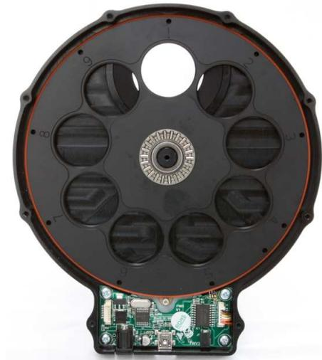
sockets exit. On the outside of the wheel near the USB socket there is a small grub screw that can be used to adjust the motor tension.
