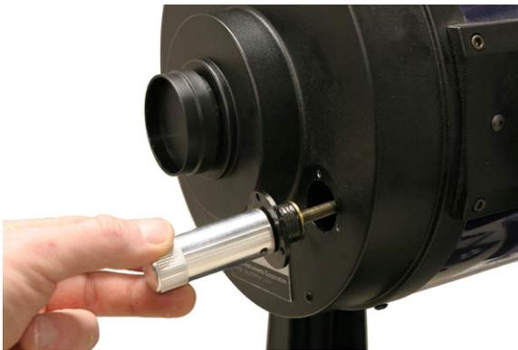
Pull the focus assembly back and tilt the outer portion to the left. This will allow the threaded shaft to slide off the right end of the small rod that holds it onto the primary mirror assembly.
