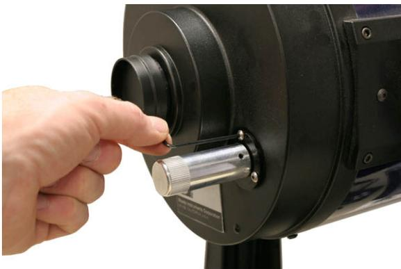
Use the 5/64" hex-head wrench to remove the three set screws holding the focus assembly in place.
