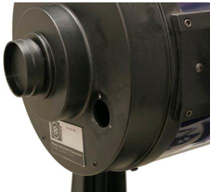
The picture above shows the tube with the focus assembly removed.
