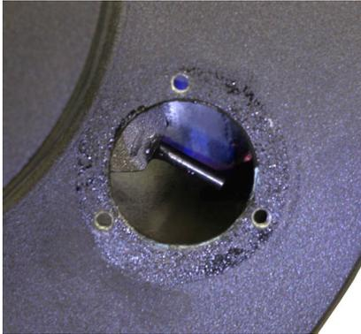
**Important:** *The focus assembly (and the new Feathertouch SCT MicroFocuser) attaches to the internal mirror assembly via a small horizontal rod. This rod points outward away from the center of the telescope tube toward the right side (when looking at the back of the scope). You must slide the focus assembly off of this rod to remove the assembly.*
