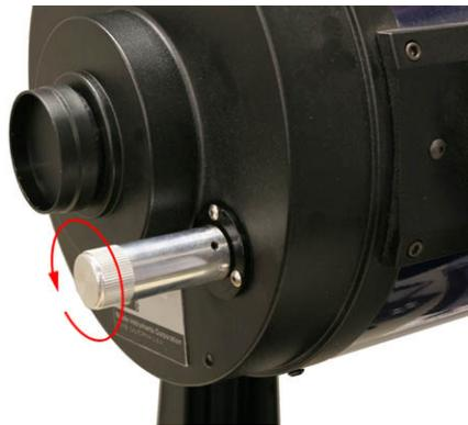
Begin by rotating the focus knob counterclockwise as far as possible to move the primary mirror all the way forward. This will make removing the focus assembly much easier.
