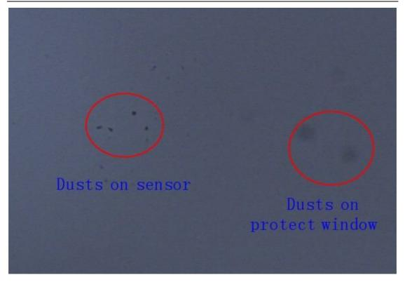
The big dim spot on the image are the shadows of dusts on the protect window.
