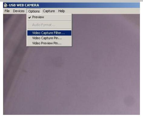
Click "Video Capture Filter" to change setting and "Video Capture Pin" to change Resolutions(you can add or remove resolutions you like).
