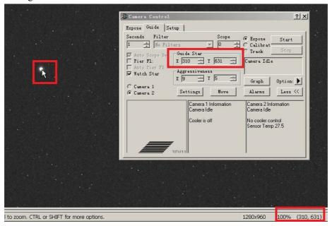
8. Click "Setting" to make sure that Autoguider output is "Guider Relays". Then MaxIm\_DL will use the ST4 port on the camera to guide. Or choose "ASCOM" driver to connect "ASICamera ST4 telescope driver" if you connect camera though WDM driver.
