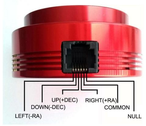
The connect cable is a 6P6C telephone-style directly connect cable.
