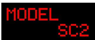
Pressing < and > buttons, the following focuser options can be set: **SC2**, **NT2**, **RT2**, **RT3**, **CUSTOM**. Pressing **MENU**, the selected focuser model is set and **BACKLIT** function will be then displayed. The software has only stored the data for the original Steeldrive. For **Steeldrive Diamond**, please select **CUSTOM** and specify a gear ratio of 0.2291. If the wrong model is set, a wrong trip will be loaded and the focuser
