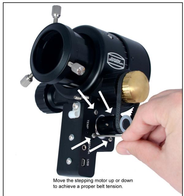
Correct tension is when the belt is tight but not tense, so that rotation of the brass knob is not impaired. The belt should yield about 5 mm when you tighten it by hand. The focuser can still conveniently be moved manually by hand, and the belt does not show any looseness or tendency to jump off the teeth. If the tension is too high, SteelDrive can't move the Steeltrack any longer, and it will stall.
