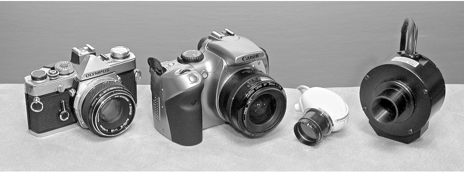
Figure 1.4. Left to right: a film SLR, a DSLR, a webcam modified for astronomy, and an astronomical CCD camera.
