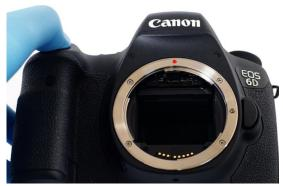
3. Select the mirror lockup item in the menu and press the shutter button to move the mirror up.
