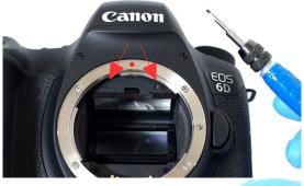
1. Loosen the two screws of the viewfinder cover using the supplied precision screwdriver.
