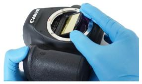
4. Insert a filter while pushing the long edge into the back of the mirror.
