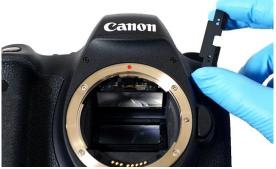
2. Remove the cover. Keep the screws and cover in a storage bag.
