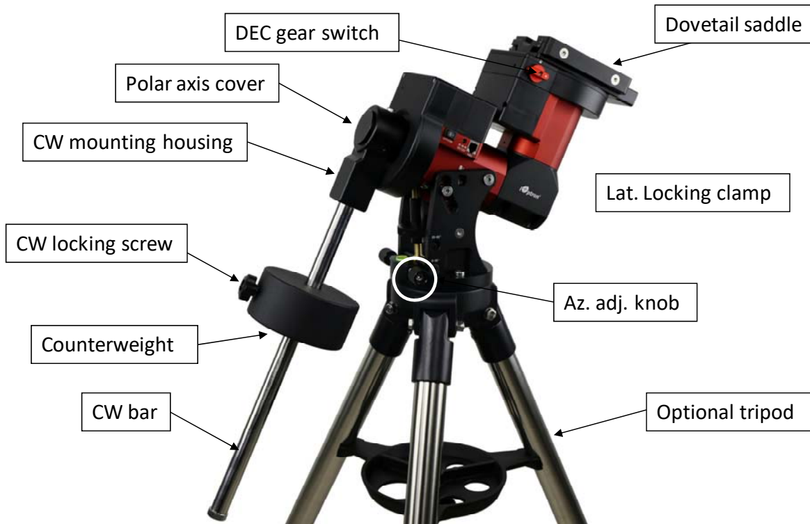
Figure 1.CEM40 mount assembly
