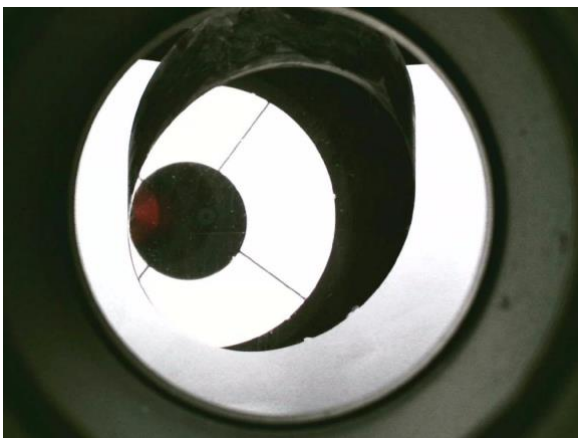
Figure 12 Not Collimated Example: secondary mirror not circular, can't see full primary mirror, etc
