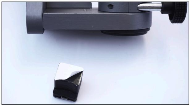
Clean the surface of the mount with an alcohol wipe, dry it and put install the reader pushing it against the tightening clamp:
