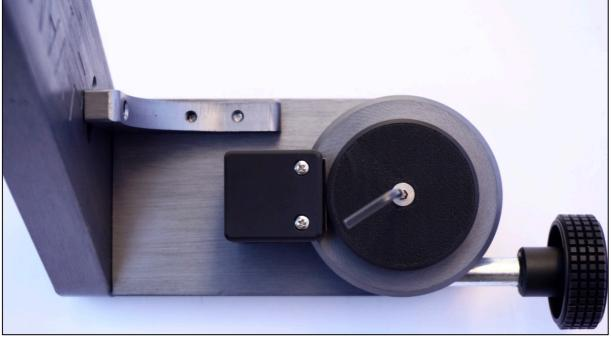
The gap between the reader sensor and the magnetic ring should be between 0.4 and 0.8mm:
