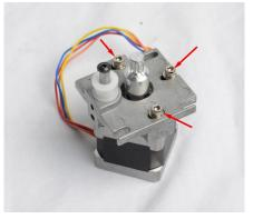
11. Slacken the 2 grub screws holding the drive gear. The gear may need to be gently levered off the end of the worm shaft. Clean any burrs left on the worm shaft made by the grub screws.
