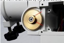
12. Fit the 47 tooth pulley on the worm shaft and 'nip' the 2 retaining grub screws. A gap of 1.0 to 2.0mm should be behind the pulley and housing.
