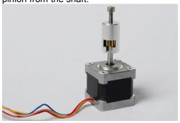
8. Fit the 9 tooth pulley on to the motor shaft and gently 'nip' the 2 x m3 grub screws. (Nip is to gently tighten with the allen key without using excessive pressure.) Do not over tighten. An approx. 5.5mm gap will be between the pulley and the raised face of the motor. This may need to be adjusted later depending on the 47 tooth pulley alignment.
