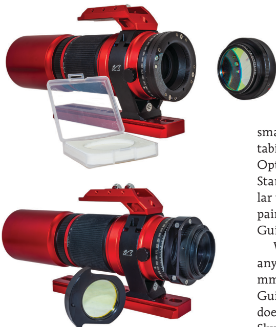
▲ Top: Two-inch filters screw into the rear adapter ring that goes between the rear adjustable cell and the 48-mm T-ring. Note the indexed camera rotator. Bottom: The after-market filter drawer from Starizona adds the convenience of quick filter changes but requires the removal of the RedCat's tip-tilt rear cell.
