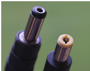
Many find the DC plug style on the right has better reliability for a stable connection.
