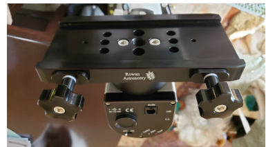
A range of saddles, the top two can do both Vixen and Losmandy. Be careful to ensure the knobs do not protrude and hit the mount at some orientations.
