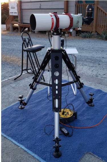
The Tri-pier (top) is supplied with adjustable feet, which may slide about on some surfaces. The modified spiked foot is made from a stainless bolt, two nuts and a wide washer. Precise leveling is more essential for Alt-Az operation and third-party leveling feet are available for the Avalon Tpod (bottom).
