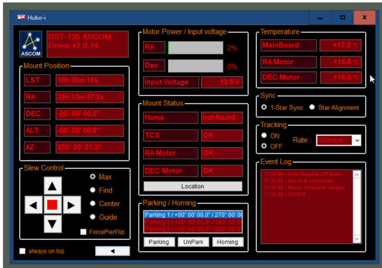
The ASCOM driver for the Rainbow pops up a Windows form to display mount information and has controls for slewing, parking, homing, tracking, and enabling sync commands.
