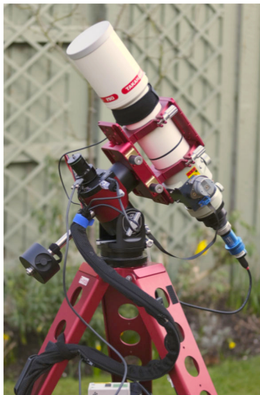
The Pegasus Power box makes for a simple one-wire connection from the mount to the ground (above). Below that, a conventional setup requires a cable bundle to prevent snagging and improve tracking consistency.
