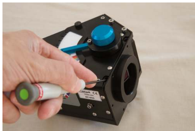
FIGURE 2.2 – Second screw of the camera adapter
