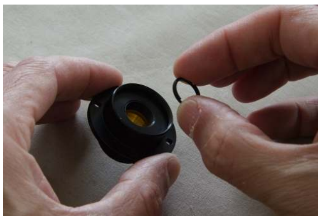
FIGURE 3.14 – Install the locking ring
