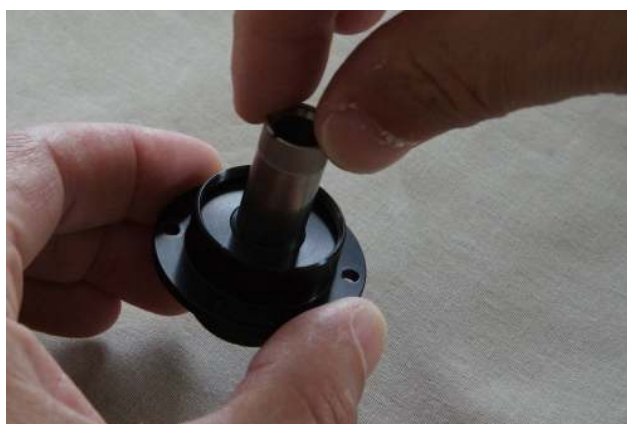
FIGURE 3.15 – Tighten the locking ring
