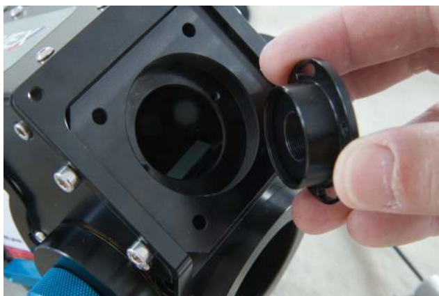
FIGURE 3.11 – Remove the external slit holder
