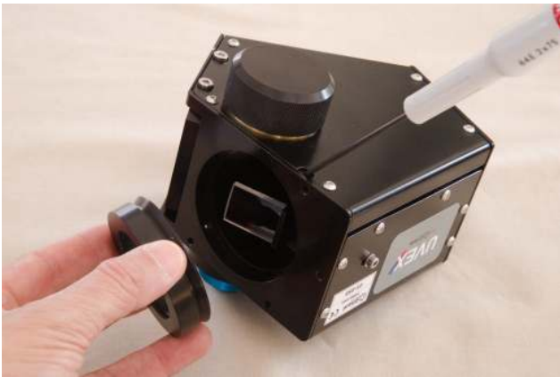
FIGURE 2.4 – Third screw of the camera adapter
