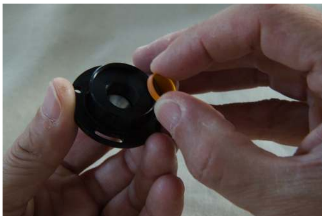
FIGURE 3.12 – Install the filter
