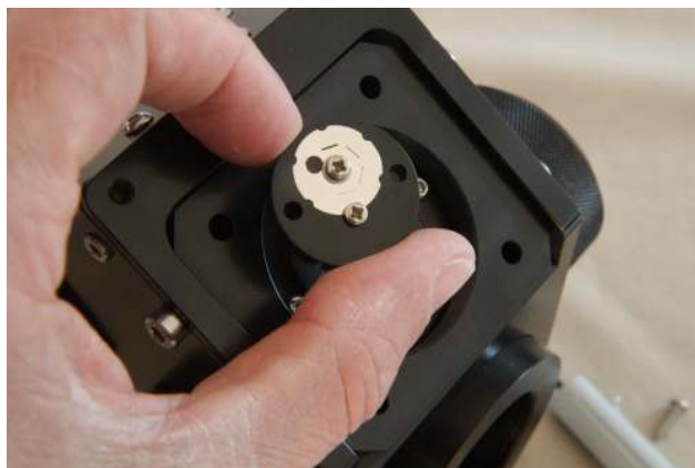
FIGURE 3.7 – Remove the slit holder
