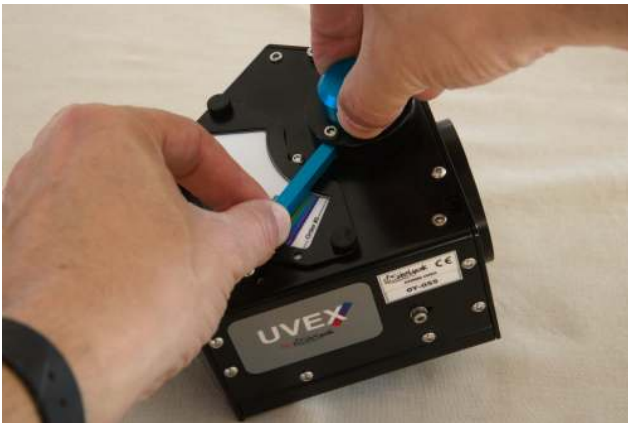
FIGURE 2.12 – Lock the grating angle
