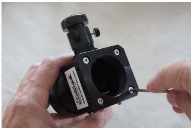
FIGURE 2.8 – Install the adapter onto guiding module
