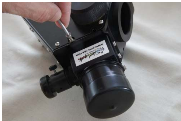
FIGURE 2.9 – Assemble the guiding module and the UVEX
