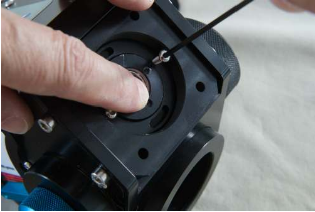
FIGURE 3.9 – Remove the external slit holder
