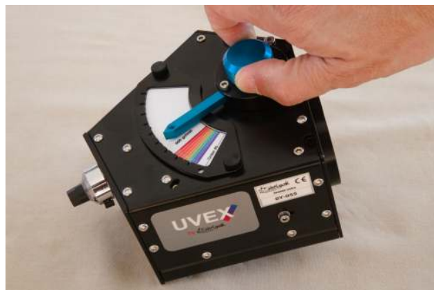
FIGURE 2.10 – Loosen the grating angle locking button
