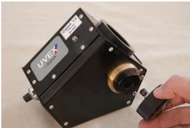
FIGURE 2.15 – Remove the grating cap
