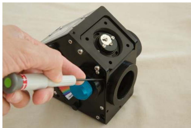
FIGURE 2.1 – First screw of the camera adapter
