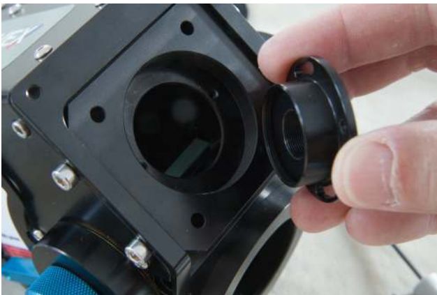
FIGURE 3.10 – Return the external slit holder to install a fiber connector
