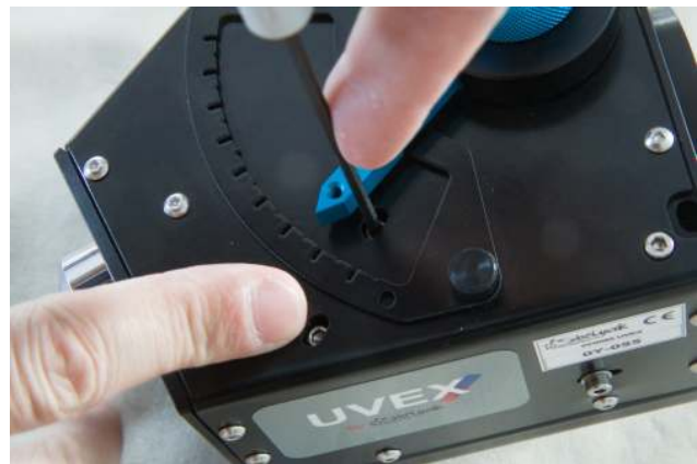
FIGURE 3.21 – Screws to control M1 tilt angle
