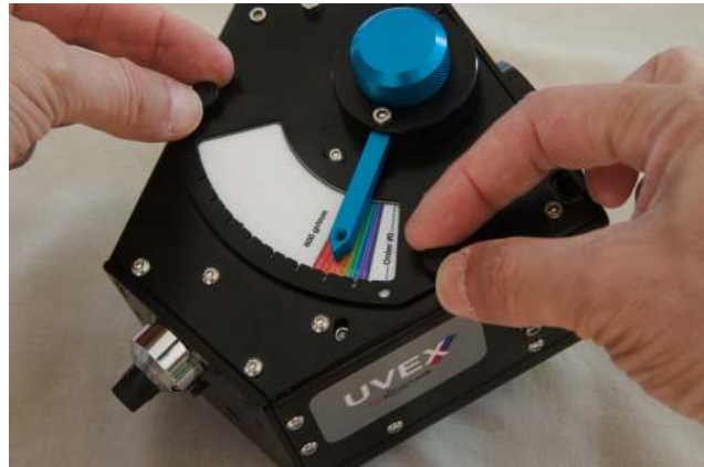
FIGURE 2.20 – Loosen the vernier screws
