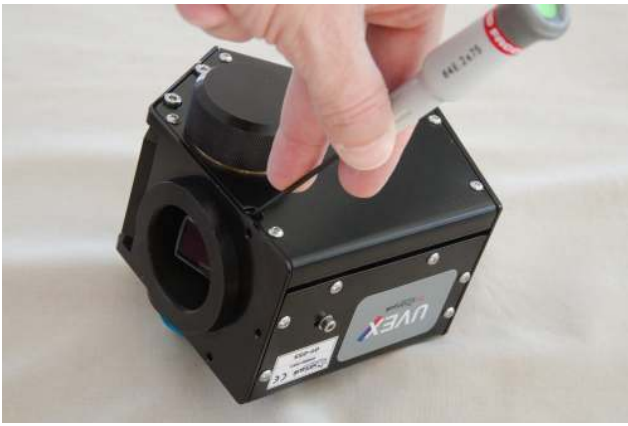
FIGURE 2.3 – Third screw of the camera adapter
