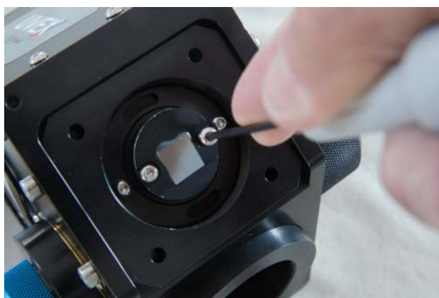
FIGURE 3.8 – Tighten the screw for the new slit
