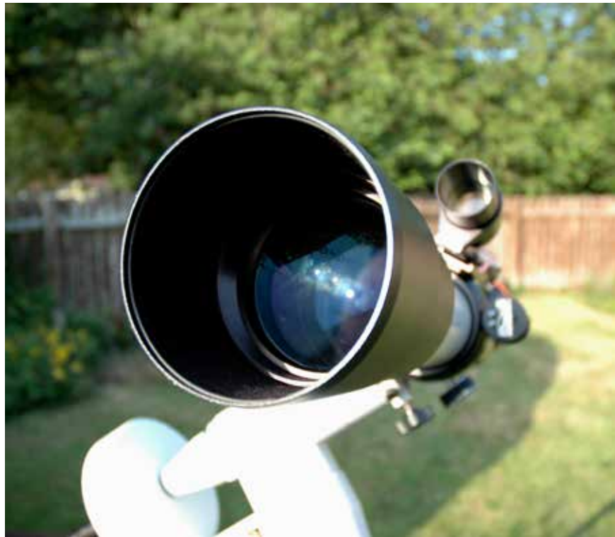
▲ Staring down the barrel of the TV-85, showing the objective lens and the dew shield up front.
