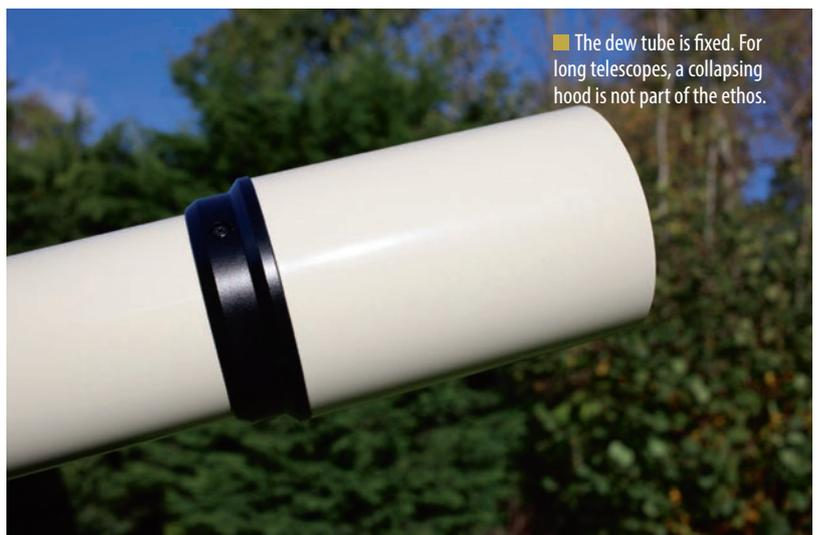
■ The dew tube is fixed. For long telescopes, a collapsing hood is not part of the ethos.
