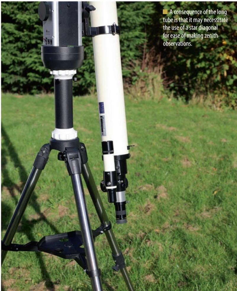
■ A consequence of the long tube is that it may necessitate the use of a star diagonal for ease of making zenith observations.
