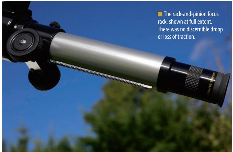
■ The rack-and-pinion focus rack, shown at full extent. There was no discernible droop or loss of traction.
