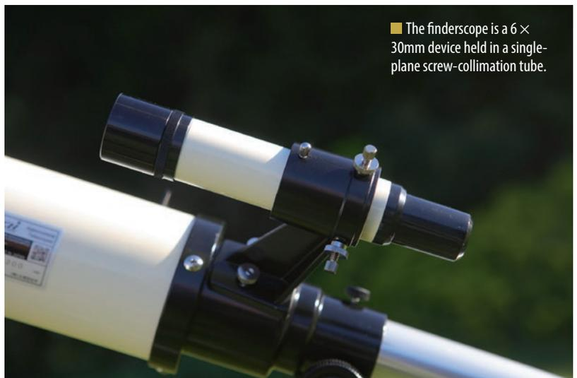
■ The finderscope is a  $6 \times 30\text{mm}$  device held in a single-plane screw-collimation tube.
