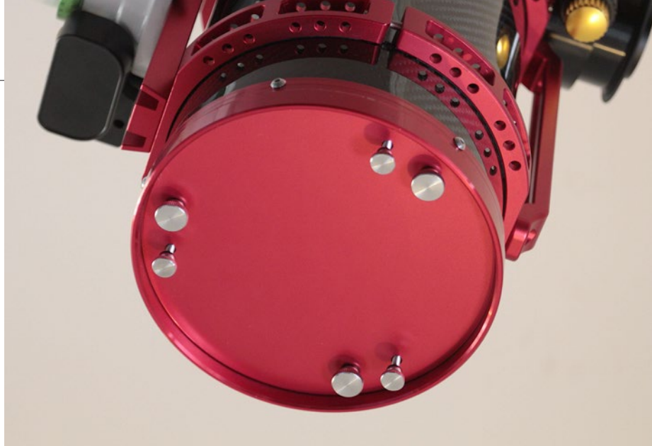
▲ The rear of the telescope that houses the primary mirror cell, and the thumb knobs used for collimating it.
