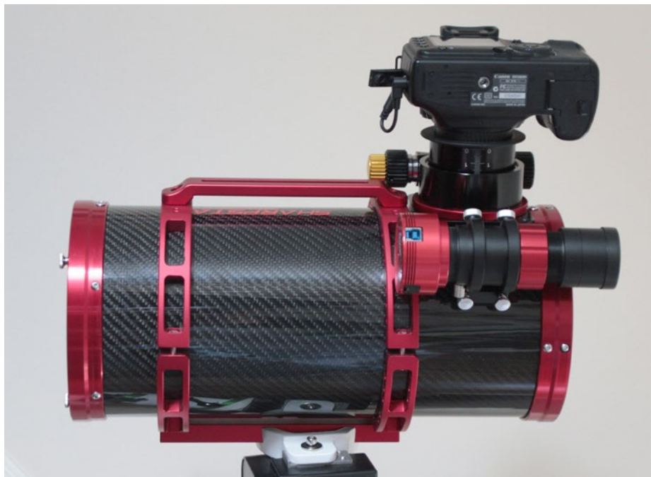
▲ A side view of the 13028HNT, with a Canon 5D DSLR (top), 30mm finder-guider and an ASI290MC guide camera.
