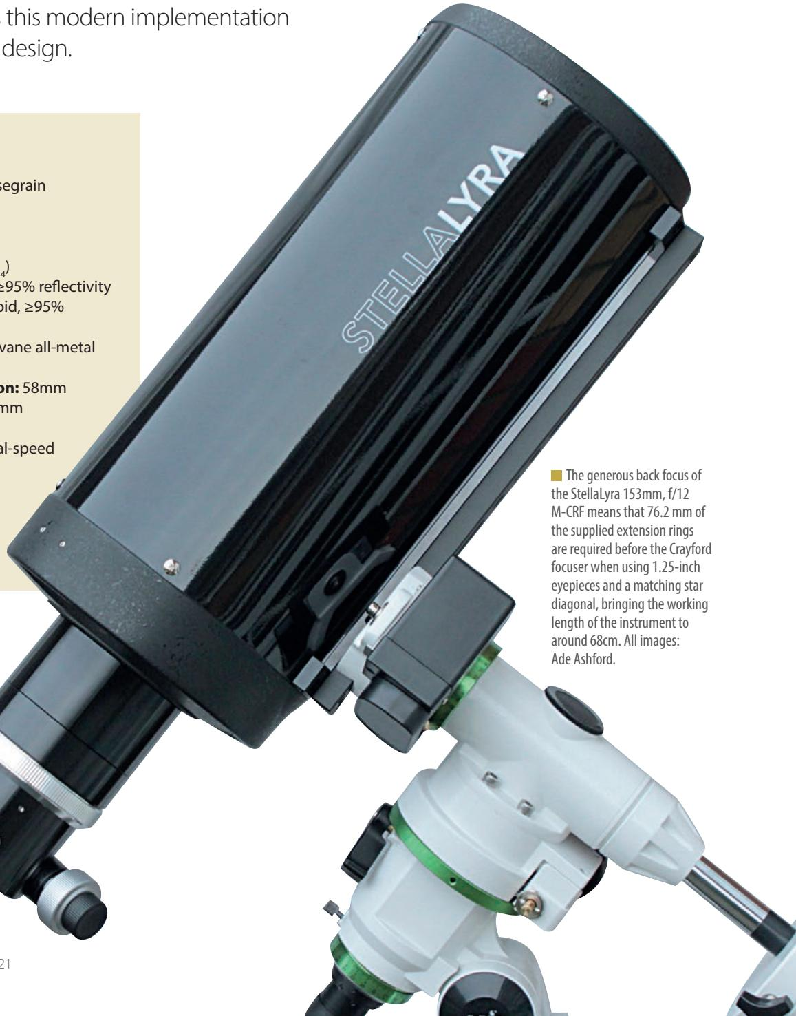
The generous back focus of the StellaLyra 153mm, f/12 M-CRF means that 76.2 mm of the supplied extension rings are required before the Crayford focuser when using 1.25-inch eyepieces and a matching star diagonal, bringing the working length of the instrument to around 68cm. All images: Ade Ashford.
