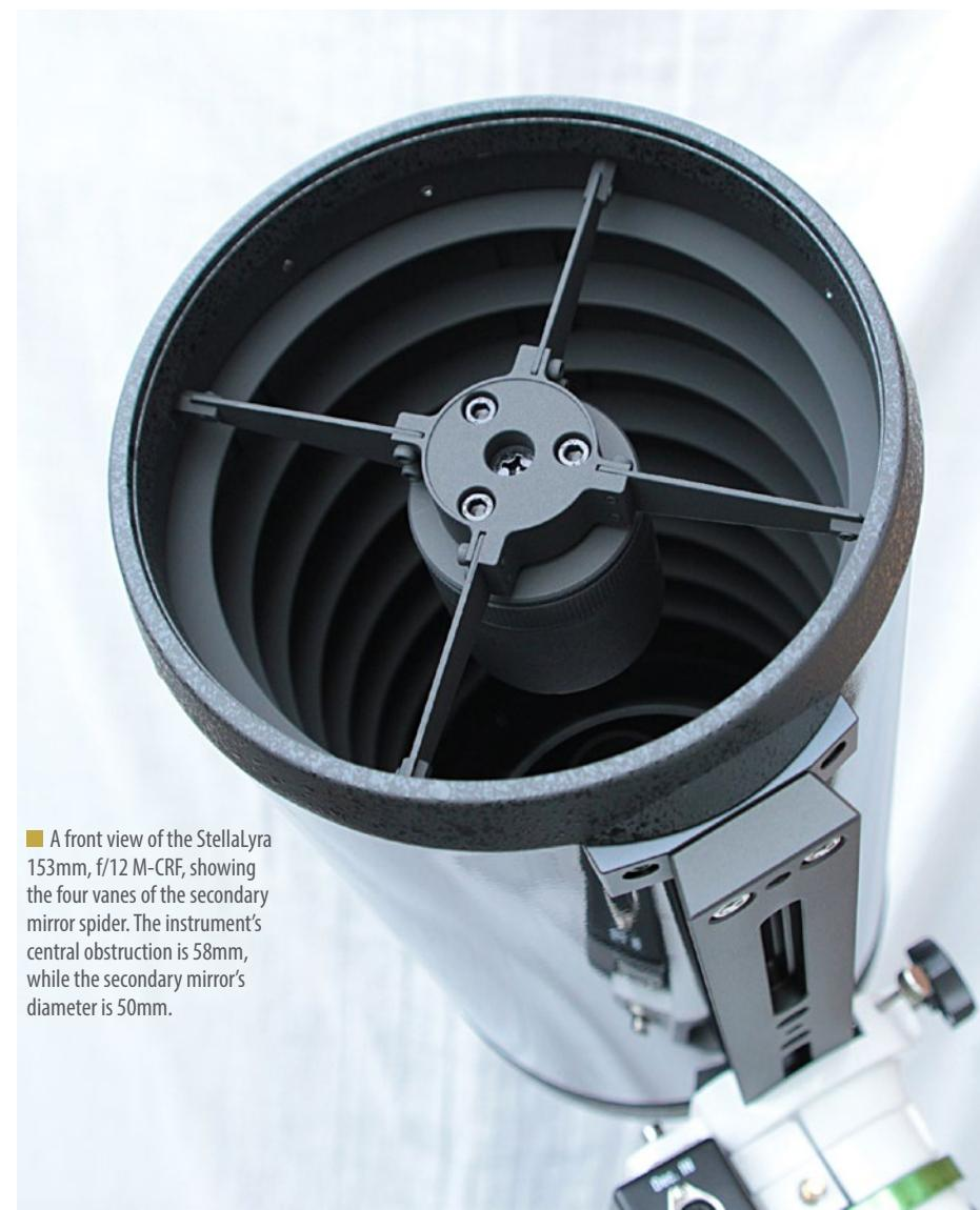
■ A front view of the StellaLyra 153mm, f/12 M-CRF, showing the four vanes of the secondary mirror spider. The instrument's central obstruction is 58mm, while the secondary mirror's diameter is 50mm.
