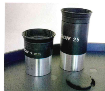
► The supplied 25mm and 9mm focal length Kellner eyepieces. Image: Ade Ashford.
