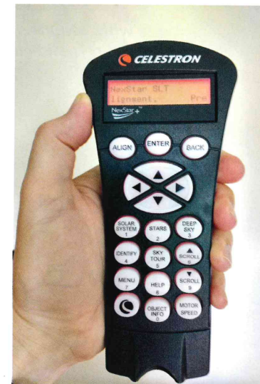
► The NexStar 6SLT is supplied with the latest NexStar+ hand controller. It incorporates a database of 40,000 objects, including planets, stars and the Messier, NGC and Caldwell catalogues. Image: Ade Ashford.
