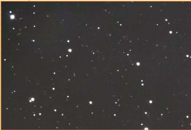
**TEST EXPOSURE** A single unprocessed 8-minute exposure of the Pleiades with a full-frame Canon 5D Mark II camera exhibits relatively little darkening of the corners from light falloff in the Esprit optics, while a blowup of the corner (left) demonstrates the pinpoint sharpness provided by the included field-flattener lens.
