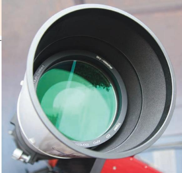
▲ A view of the 152mm (six-inch) lens assembly. The green colouration is produced by the lens' high-transmission coatings. Just visible are a few of the interior baffles. The large retractable dew-shield is held in place with two thumbscrews and did a very good job of withholding dew formation. At no point during the review period, even on damp evenings, did dew ever form on the objective lens.
