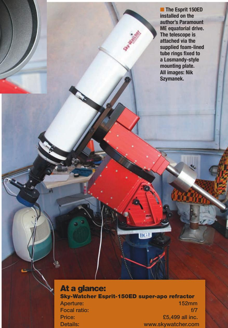
■ The Esprit 150ED installed on the author's Paramount ME equatorial drive. The telescope is attached via the supplied foam-lined tube rings fixed to a Losmandy-style mounting plate. All images: Nik Szymanek.
