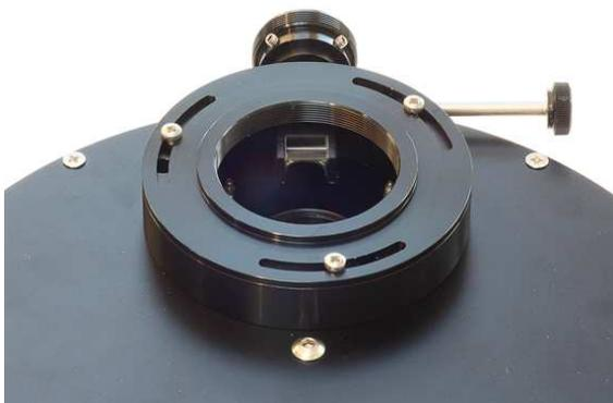
Installation on the filter wheel casing was simple using the three cheese-head M2.5 x 5mm bolts supplied and the whole construction felt very secure indeed.
